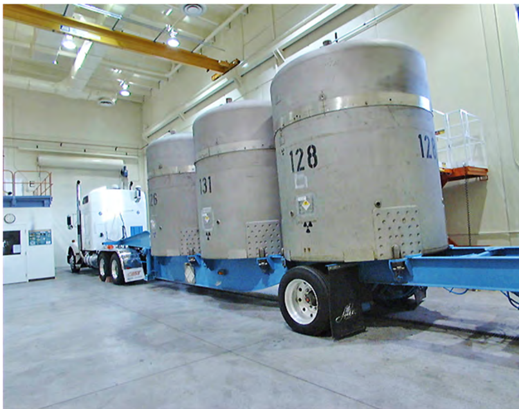
Three TRUPACTs with TRU waste waiting to leave for WIPP. Courtesy LANL
